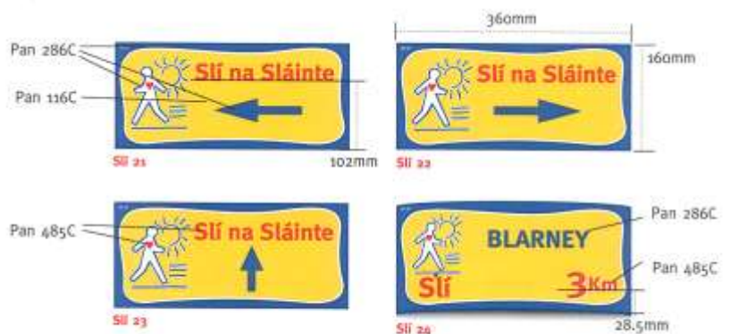
6. Urban Directional Signs – located at junctions in urban areas. Normally attached onto existing posts with banding but can be attached onto new 2.4mtr posts.
