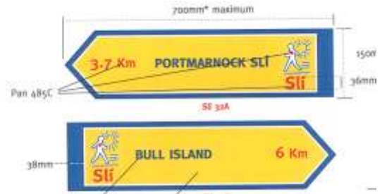
3. Finger Posts – can be attached onto existing posts or onto a new 3.4mtr pole.
